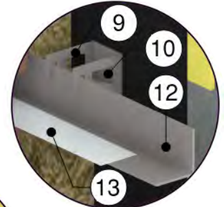
FERO FAST Thermal Bracket System
