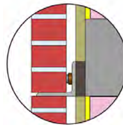
Shelf angle outboard of R-5 insulation
