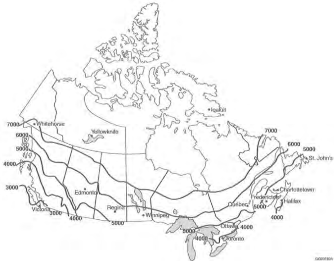
Fig. 2.3.1 Canadian heating degree days (HDD °C) and climate zone divisions, as per the 2011 National Energy Code for Buildings. (Reproduced with the permission of the National Research Council of Canada.)
