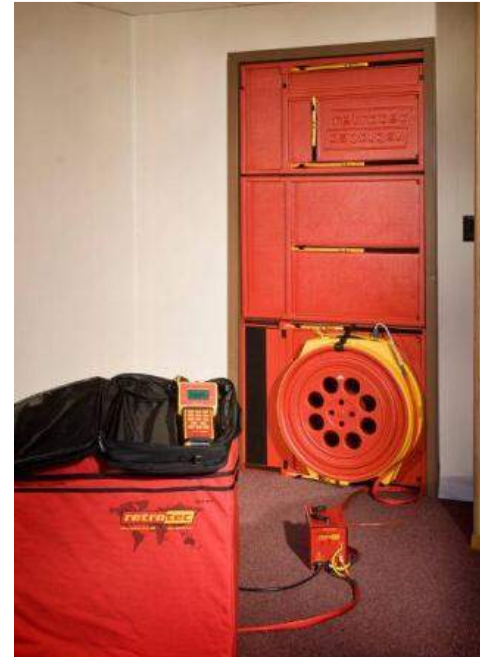
Fig. 5.2 Fan door equipment setup (photo courtesy of Retrotec Energy Innovations Inc, Vancouver, BC)
