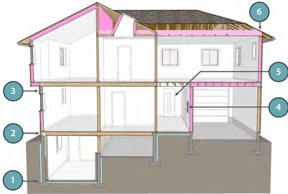
Figure 2: Typical Problem Areas for Insulation Continuity
