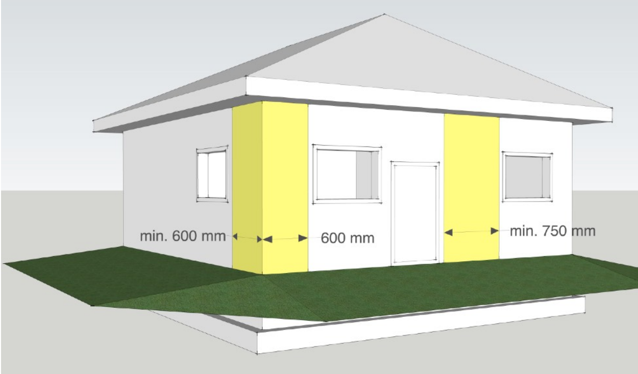
Minimum length of braced wall panels when connecting to intersecting braced wall panels, and minimum panel length in the field of the wall. xi
