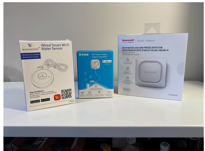
Some leak detection devices are WiFi enabled and can send notifications directly to your email or smartphone app if a water leak is detected
